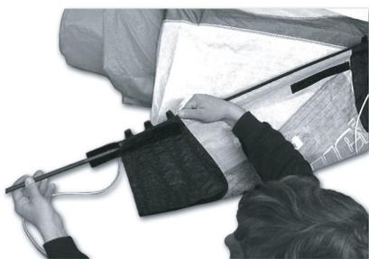
9. Install Batten in Pocket provided UNDER the Bridle Pocket
