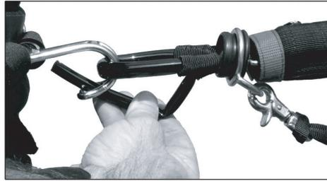
2. Bend "Chicken Bone" and Feed into Spreader Bar Hook.
